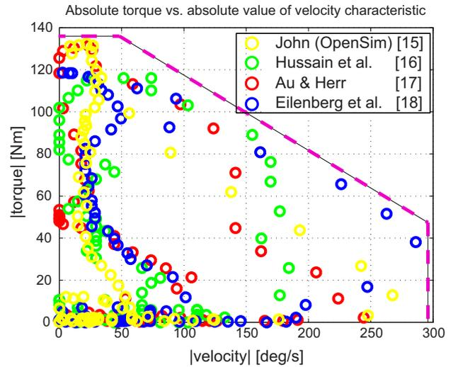
Fig. 4. The torque-velocity characteristic during walking for a 75 kg subject. To emulate normal human ankle joint, the torque-velocity characteristic of an actuator must be above the purple dashed line.
