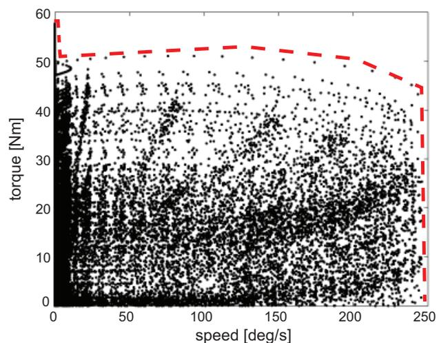
Fig. 7. The torque-velocity scatter plot obtained from the parallel-cascade stiffness model simulation. To emulate the ankle joint, the torque-velocity curve of an orthosis actuator must be above the red dashed line.
