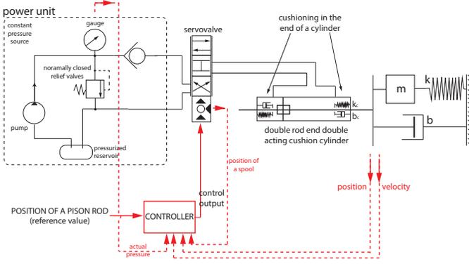
Fig. 1. Overview of the modeled system
