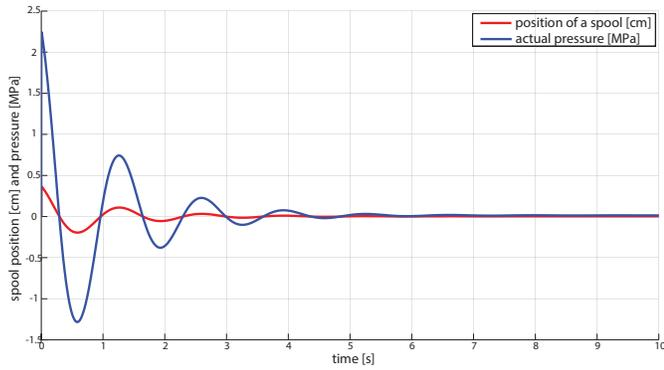
Fig. 2. Time history of position of a valve's spool and differential pressure
