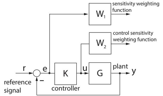
Fig. 4. Augmented plant used in the loop-shaping framework
